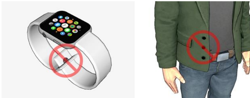
<Figure 15. Magnetic ornaments may cause the perturbation of the magnetic field>
